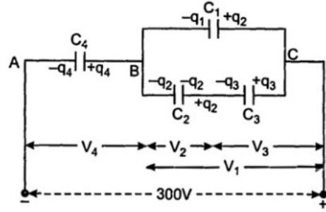
$\therefore C_1 = C_4 = 100 \text{ pF} = 10^{-10} \text{ F}$
