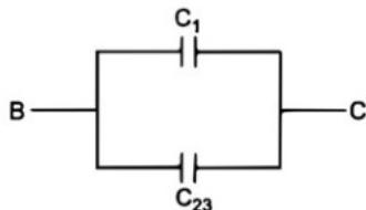
$$\begin{aligned} \frac{1}{C_{23}} &= \frac{1}{C_2} + \frac{1}{C_3} \\ \text{या } \frac{1}{C_{23}} &= \frac{1}{200} + \frac{1}{200} \\ \text{या } \frac{1}{C_{23}} &= \frac{2}{200} \\ \text{या } \frac{1}{C_{23}} &= \frac{1}{100} \end{aligned}$$
