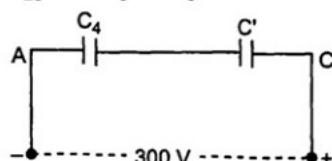
$$\begin{aligned} C' &= C_{23} + C_1 \\ \text{या } C' &= 100 \text{ pF} + 100 \text{ pF} \\ \text{या } C' &= 200 \text{ pF} = 2 \times 10^{-10} \text{ F} \end{aligned}$$
